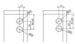
Rear drilling pattern for active safety version. Two possibilities.
