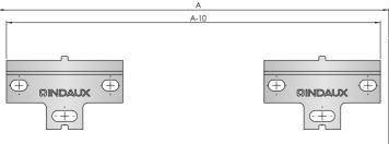
Side adjustment 10mm. A: Distance between cabinet sides. \*The screws must have ridged head.
